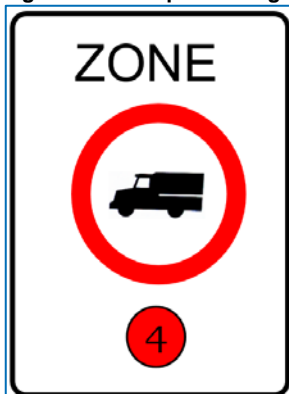
Figure 2.2 Example LEZ sign showing that lorries with pollutant class 4 or higher are permitted to enter.
