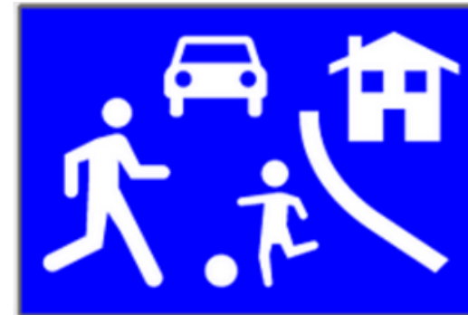
e) Pedestrian Priority Zone entry sign
