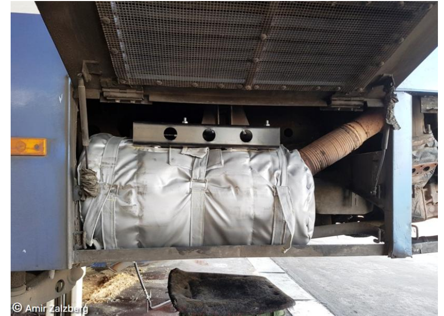
A subsidised diesel particulate filter installed on a truck in Jerusalem
